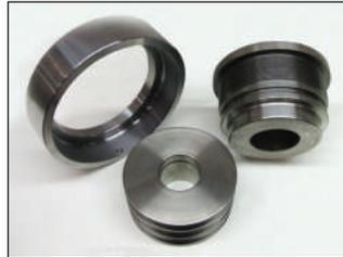
Pistons and glands are made of some of the highest quality ductile iron available. Hard chrome plated steel is standard material for the rod (shaft). Other materials, such as nitrided (which has excellent dent and corrosion resistance), or induction hardened are available.
